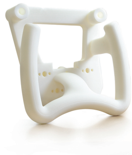
BMW's jigs and fixtures department used a Fortus® 3D Production System to manufacture assembly tools. This tool is used to affix the rear name badge.
