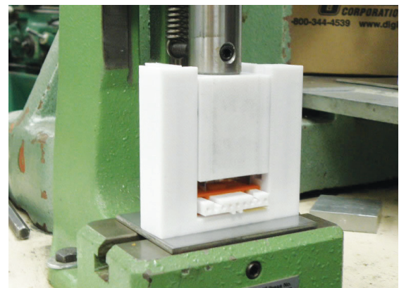
An operator at Xerox modified 350 connectors in about an hour on this toggle press.
