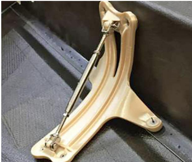
Manufacturing tool 3D printed using ULTEM™ 9085 resin enables Indaero to produce complex shapes that perfectly fit the curvature of aircraft panels not possible with traditional aluminum tools.
