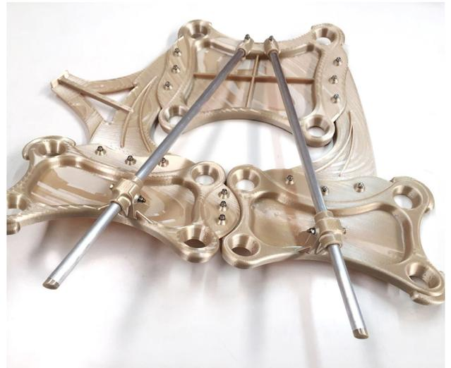
Indaero redesigned and 3D printed a tool nine kilos lighter than the traditionally manufactured tool.
