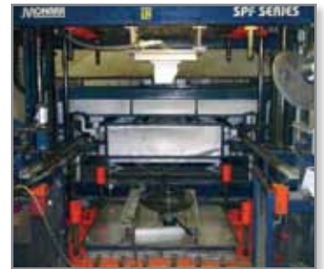
FDM tool mounted in thermoforming machine
