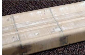
Figure 27: When using fillers, sand the surface until a striping pattern appears.
