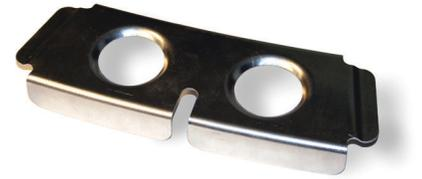
Finished product hydroformed from an FDM tool.
