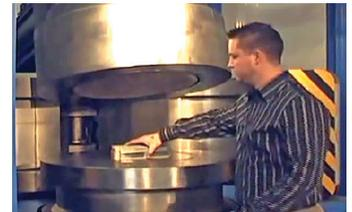
Figure 30: Blank and form block are placed in hydroforming press.
