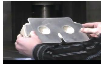
Figure 29: Sheet metal blank on form block.
