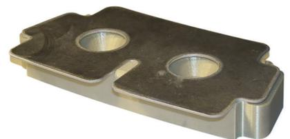
Figure 3: FDM ULTEM 9085 tool (with sheet metal blank) has exceeded 400 cycles.
