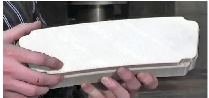
Figure 10: intensifier (top component of tool set) reduces forming pressure. See Figure 11 for reference.
