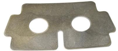
Figure 2: Sheet stock up to 0.090 in. (2.29 mm) has been formed.
