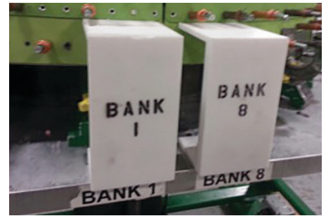
3D printed templates inspect contoured panel edges
