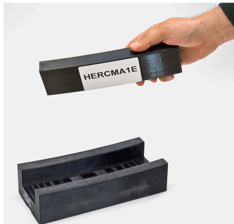
3D printed forming tool in Stratasy Nylon 12.
