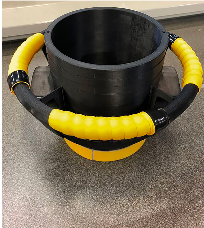
Final, 3D printed ECS duct adapter designed to cool aircraft while on the ground. 3D printed in Stratasys FDM Nylon 12 on the Fortus 450mc.
