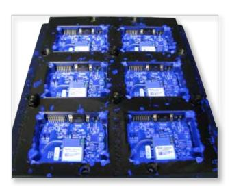
The application is jig and fixture making — which also includes gauges, organizational aids and other manufacturing devices. AM produces these tools by adding material in an automated, layer-by-layer process rather than removing material with a cutter or forming it in a mold.
