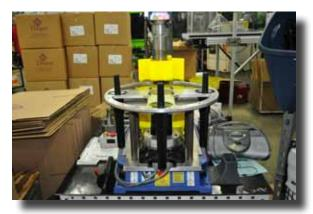
At Thogus / rp+m, production aids, such as the yellow safety shield and gray diverter (foreground), have proliferated with additive manufacturing.
