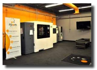
Three of rp+m's FDM additive manufacturing machines.
