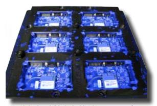
FDM hybrid mask (black) shields PCB components from conformal coating (blue under ultraviolet light).
