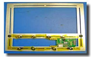
Machined carrier with manually applied tape for masking.
