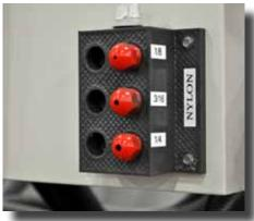
Injection molding nozzles organized in an additvely manufactured work holder to make them accessible to press operators.
